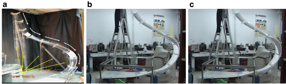
Fig. 1 (a) A twisted channel used in experiments (Pudasaini et al. 2008): Upper part is straight and inclined at 45°; the middle part is twisted, and the lower part consists of transition and runout zones merging into the horizontal plane. Both the upper and lower parts are cylindrical with radius of 9.7 cm. Total length of the channel = 600 cm, upper straight part = 85 cm, middle twisted part = 365 cm, lower transition part = 50 cm and horizontal flat part = 100 cm. (b) Granular avalanche (of quartz sand) showing the front of superelevated mass induced by the curvature and torsion of the channel. (c) The main body of superelevated avalanche. The avalanching mass is seen in a relatively grey colour around the main bending, whereas the channel is in light grey. The downward arrows in panels B and C indicate the avalanche positions
