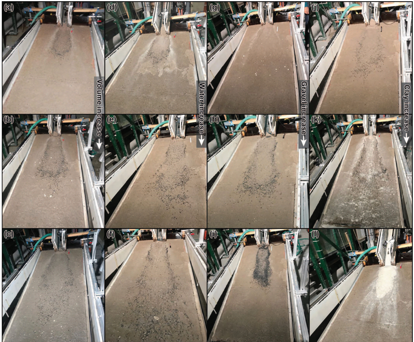
Fig. 9.—Photograph highlighting grain-size sorting in selected subaqueous debris flows. The coarse-grained gravel particles have a black color, the sand is brown, while the clay has a white color. A–C ) Debris flows with an increasing volume and mass of 3.5 kg (exp. 2 in Supplemental Table 1), 8.0 kg (exp. 10), and 11.0 kg (exp. 13), respectively. D–F ) Debris flows with an increasing volumetric water content of 40% (exp. 24), 50% (exp. 25), and 60% (exp. 30), respectively. G–I ) Debris flows with an increasing gravel content of 0% (exp. 32), 39% (exp. 35), and 64% (exp. 39), respectively. J–L ) Debris flows with an increasing clay content of 0% (exp. 42), 11% (exp. 45), and 29% (exp. 50), respectively. Boundary conditions for the subaqueous flows shown here match those shown in for subaerial flows shown in Fig. 8. Note the changing perspective between photographs. See Supplemental Table 1 for experimental details.
